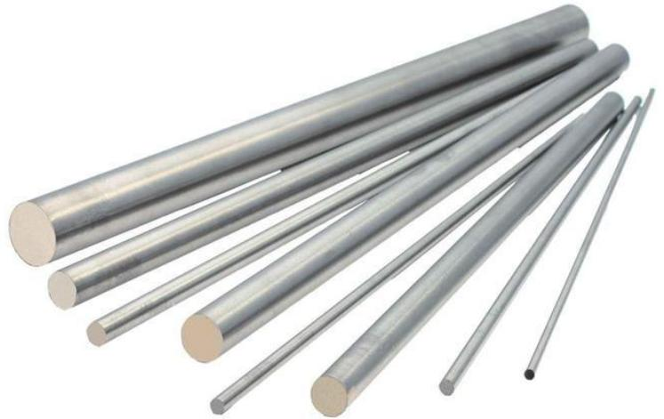
**YG10X** Use widely, with good hot hardness. Suitable for milling and drilling general steel under 45 HRC and Aluminum, etc at a low cutting speed. Recommend use this grade to make the twist drills, end mills, etc.
